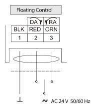
NOTE: To avoid excessive wear or drive time on the motor, use a controller and/or software that provides a time-out function to remove the signal at the end of rotation (stall).
