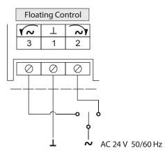
NOTE: To avoid excessive wear or drive time on the motor, use a controller and/or software that provides a time-out function to remove the signal at the end of rotation (stall).
