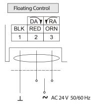
NOTE: To avoid excessive wear or drive time on the motor, use a controller and/or software that provides a time-out function to remove the signal at the end of rotation (stall).
