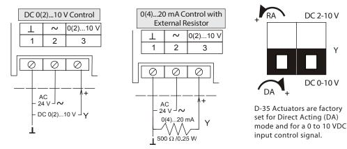
NOTE: To avoid excessive wear or drive time on the motor, use a controller and/or software that provides a time-out function to remove the signal at the end of rotation (stall).
