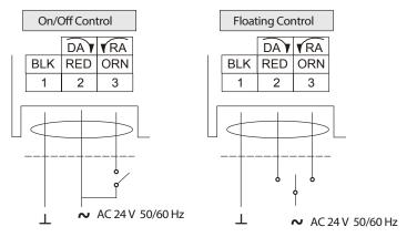
NOTE: To avoid excessive wear or drive time on the motor, use a controller and/or software that provides a time-out function to remove the signal at the end of rotation (stall).
