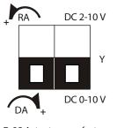
D-35 Actuators are factory set for Direct Acting (DA) mode and for a 0 to 10 VDC input control signal.
