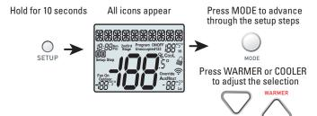
Technician Setup is for diagnostic and testing purposes and is intended for use by a qualified technician. See page 14 for more detailed instructions.
