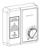
vided with the unit. The dehumidistat provides high-speed ventilation when the indoor humidity level exceeds the setpoint. This low voltage control connects to the HRV micro-processor board by two wires. See the wiring diagram on page 16 of this manual.
