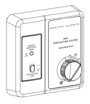
The HRV remote control (72X53) includes an ON/OFF switch, a dehumidistat, and a \*service reminder light. The low voltage control is connected to the HRV micro-processor board by three wires. This control satisfies many building code requirements. See the wiring diagram on page 16 of this manual.
