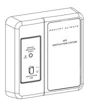
The ERV remote control (72X54) includes an ON/OFF switch and a \*service reminder light. The low voltage control is connected to the ERV micro-processor board by two wires. This control satisfies many building code requirements. See the wiring diagram on page 17 of this manual.
