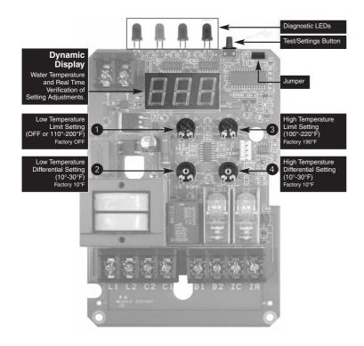
**NOTE:** Be careful not to select overlapping temperature settings. For example: If the HIGH TEMPERATURE LIMIT is set at 190°F with a HIGH TEMPERATURE DIFFERENTIAL set at 20°F, then the LOW TEMPERATURE LIMIT needs to be set at 170°F (190°F - 20°F = 170°F) or below.
