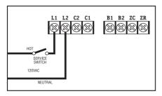
**STEP 1** Connect 120 VAC Hot to terminal **L1**. Connect 120 VAC Neutral to terminal **L2**. Disconnect means and overload protection as required (provided by others).
