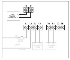
**STEP 4** Connect the thermostat to T and T.
