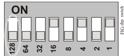
Figure 9: Device Address Switches Set to 21
