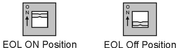
Figure 10: EOL Switch Positions
