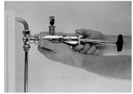
7. Holding the changer so that is does not turn, turn the bonnet out of the chamber.
