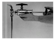
4. Check that the drain cock is closed and that the bonnet of the outer chamber of the changer is assembled securely. Turn the changer handle counterclockwise at least 3 full turns to ensure that the insert is free. Pull out on the changer handle to clear the ball valve.
