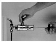
5. Close the ball valve by turning its handle so that it is across the axis of the changer.
