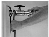
2. Place the socket of the insert changer onto the valve insert. Press in the stem handle of the tool to ensure a firm engagement.
